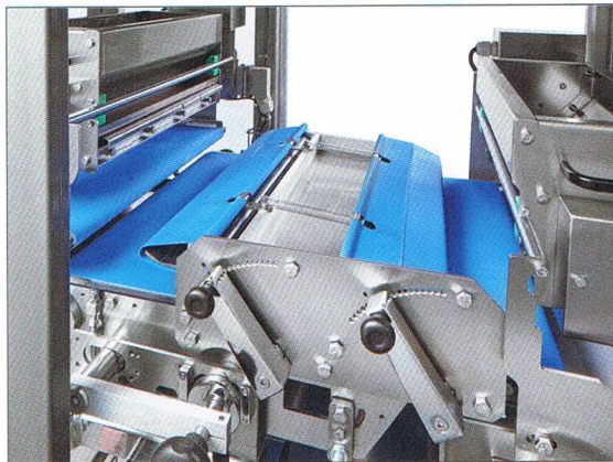
Long-loaf moulding table before the stamping unit.
