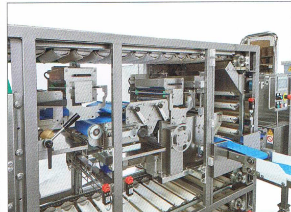
Flour duster before the stamping unit and/or before the moulding station.
